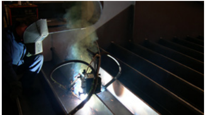
Tortuga with two torches for welding of bridge beams
