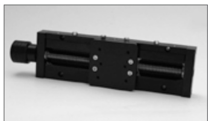
SMMD 160-1 one-axis slide, stroke 160 mm Aluminium machined body, steel screw, bronze nut, brass dovetail slider with adjuster, knob in knurled aluminium
