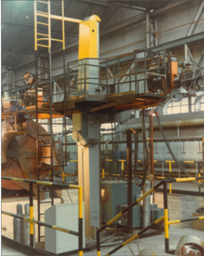
ET-250: SAW of forged elbows
