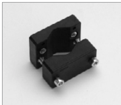
SMMD-PT, torch clamp Made of synthetic material, suitable for torch Ø 18 to 40 mm, it can be fixed in horizontal or vertical position
